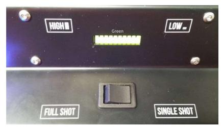
The green bar represents the capacity of the battery in the gun. When fully charged the Bar will be completely green. When the battery is depleted only the first led on the bar will flash red.
