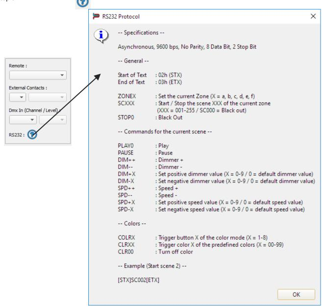
Connect the RS232 transmitter to the interface RS232 and GND pins and send the dedicated ASCII commands lines that you need.
