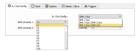
The Stand Alone mode offers up to 512 DMX IN channel triggers and up to 255 DMX trigger values per channel. By selecting a scene in the list, it's possible to choose the channel number and the DMX value to trigger the scene. The scene will play when the value of the DMX channel is reached or exceeded.
