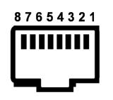
Front view of the interface RJ 45 connector
