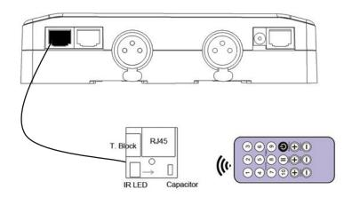
In the software go to Stand Alone Mode and use the Triggers options to assign a remote button to a scene. Standalone mode offers up to 10 triggers with the Infrared remote.
