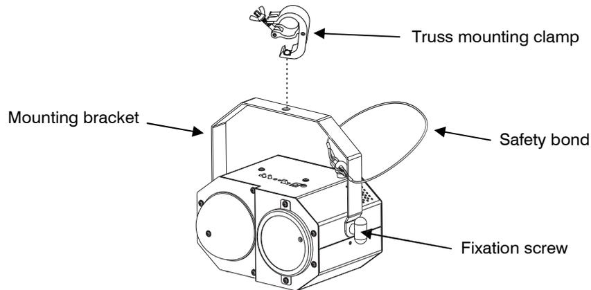
This product is designed for overhead rigging to a wall or ceiling with the mounting bracket. It can also be fastened to a truss using appropriate clamps. To align the unit, release the fixation screws at the mounting bracket, adjust the desired inclination angle and retighten the fixation screws.
