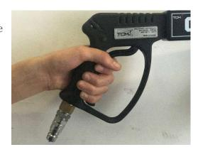
Turn the safety catch downward to lock the handle after use.
