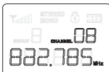
Use the button ▲ or ▼ to select new group (0-9) and confirm with **SET**. On the display, "**CHANNEL**" and the current channel number will now be flashing.
