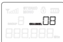
Switch on the receiver by turning the **level control** from the left stop. The display will show the receiving frequency adjusted last and the corresponding group and channel number. Unfold the front cover and press the button **SET**. The setting menu will be called with menu item "**GROUP**" selected. On the display, "**GROUP**" and the current group will be flashing.
